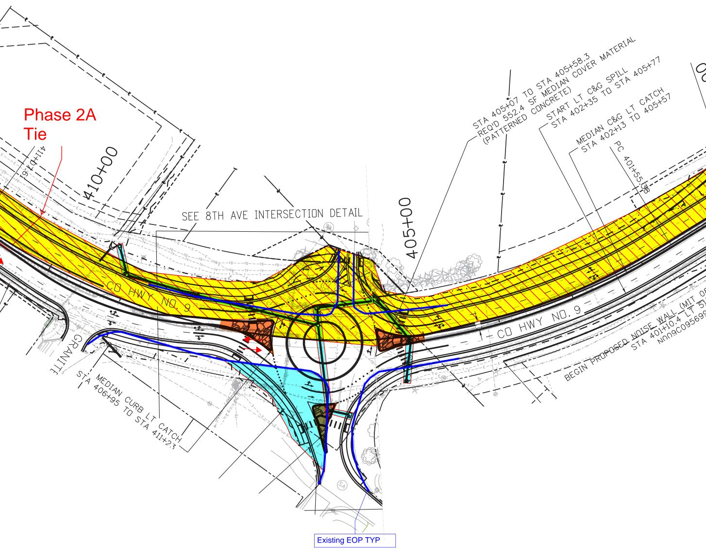
Phase 2A-1 -Shift all traffic through intersection to SB side @ main. -Finish NB to end of project. **Duration: June-July**
