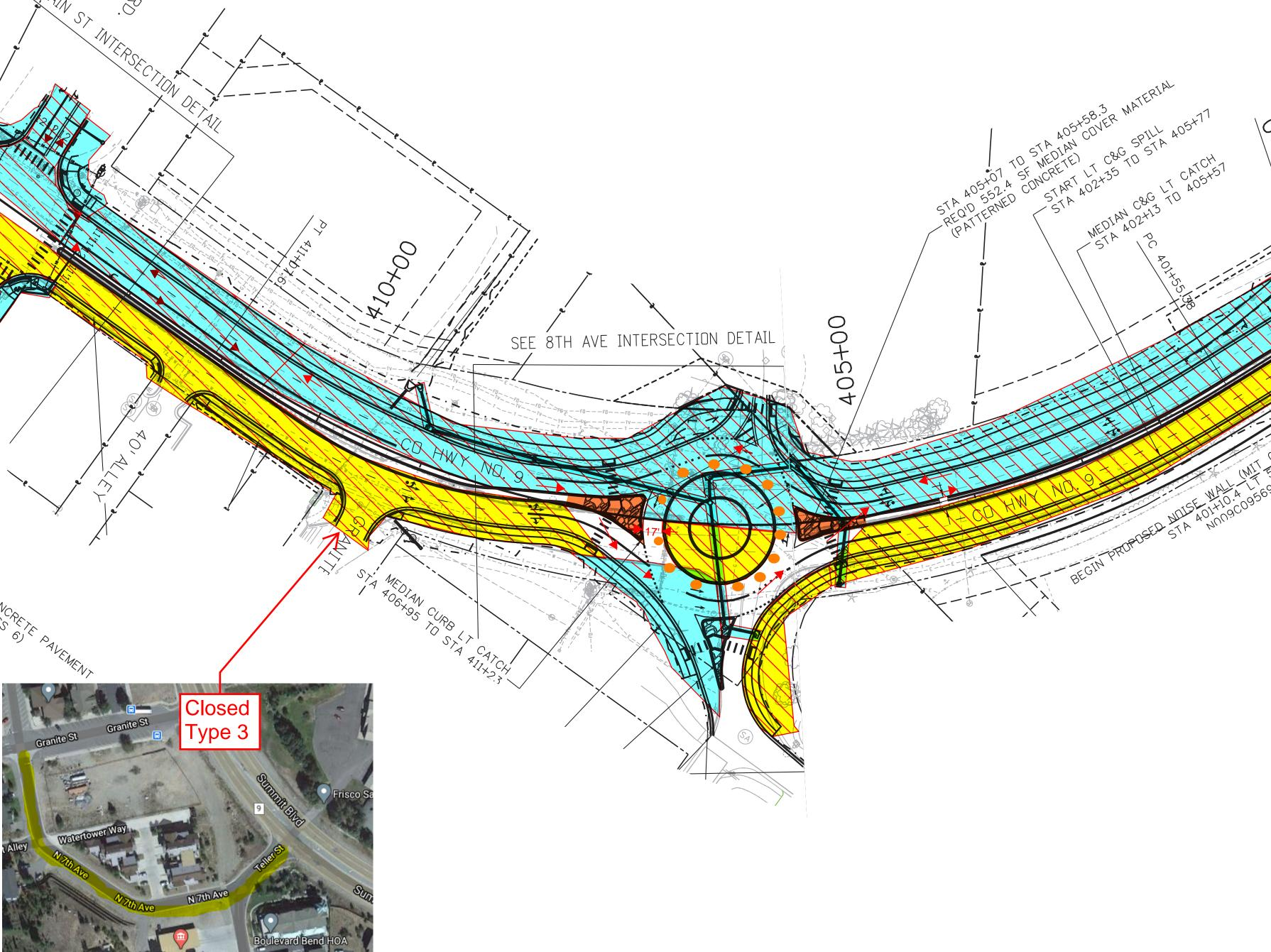
Phase 2B -Open Temp Roundabout -Shift Traffic to NB side of SH-9 -Mill & Pave Main Night/Fast track. Duration:July-September
